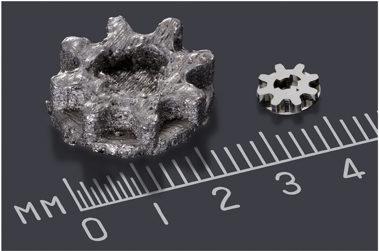
Fig. 5. Optical image of an enlarged SLM-produced gear (left) and a MICA Freeform produced gear.
